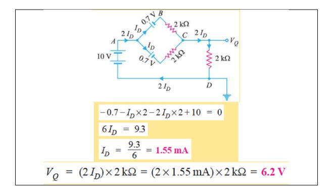
6- Determine current through each diode in the circuit shown. Use practical model. Assume diodes to be similar .
