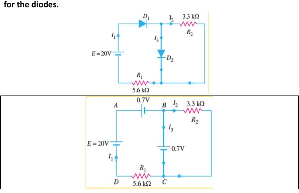
The voltage across  $R_2$  (= 3.3 k  $\Omega$ ) is 0.7V.
