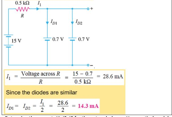
7- Determine the currents I1, I2, I3 for the network shown. Use practical model for the diodes
