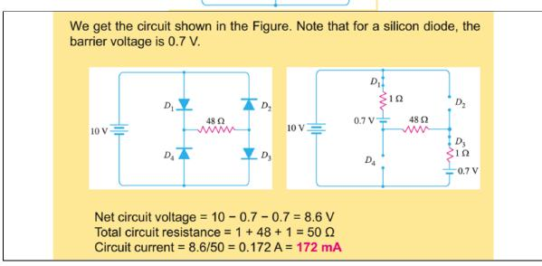
4- Determine the current I in the circuit shown in the Figure. Assume the diodes to be of silicon and forward resistance of diodes to be zero.
